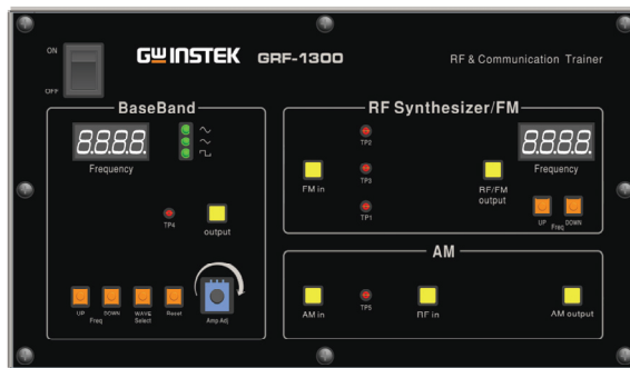
Figure A-1. The GRF-1300 control panel
